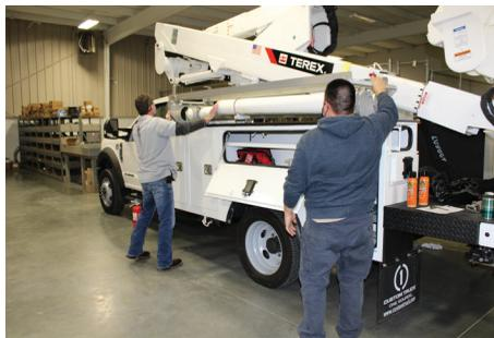
*Operations Manager Jody Parker and Maintenance Technician Ruben Chavez install a tube that holds a hot stick on the co-op's new service truck.*
