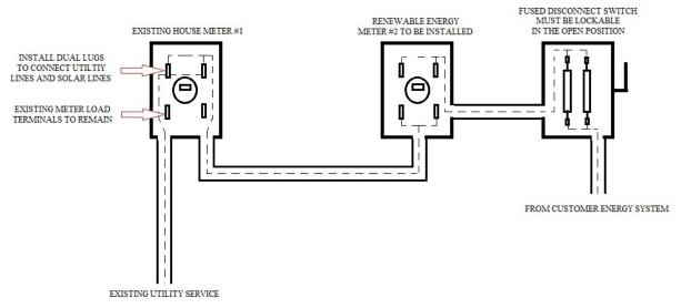
WIRING AND RACEWAYS TO BE SIZED AND INSTALLED IN ACCORDANCE WITH ALL APPLICABLE LOCAL, STATE, AND NATIONAL CODES
